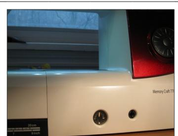
This circle has a slot in the middle for a screwdriver or a coin, and a "plus" sign and a "minus" sign. To resolve the appearance of the stitch you simply turn to + or -, test sew, and if not correct try the other setting. When reverting back to another stitch change the setting back to midpoint.
